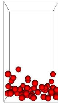
Figure 1: A snapshot of a suspension with 50 spheres. This figure is a typical example of a system that has reached a steady state: all particles have fallen to the ground leaving most of the simulation volume being free of particles [19].
