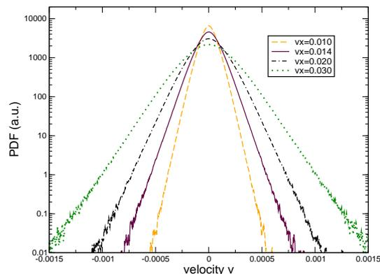
Figure 5: Probability distribution function of the particle velocity in vertical direction. The data corresponds to the snapshots in figure 4. The tails are exponential and follow a law as given by equation 9.
