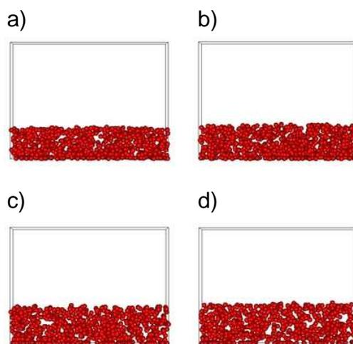
Figure 4: A snapshot of a suspension with 768 spheres after 6.25 million timesteps and varied shear rate used to gain statistics of particle velocity distributions. Shear rates are  $v_s=0.010$  (a),  $v_s=0.014$  (b),  $v_s=0.02$  (c),  $v_s=0.03$  (d) (in lattice units). It can be observed that the height of the occurring sedimentation layer depends on the shear rate.
